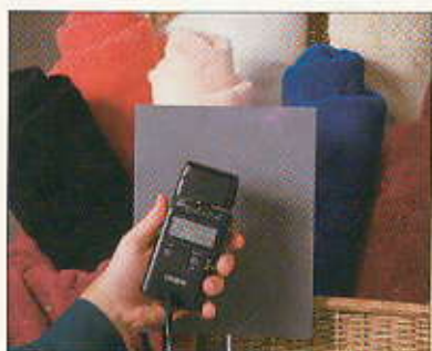
The meter position is too close and in the light path, casting a shadow on the reading area.
