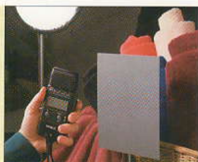
The meter is too far from the subject, causing stray light to spill on the meter.
